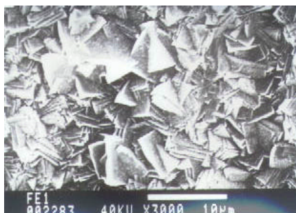
Figure 2 The SEM image of the zeolite NaA membrane
